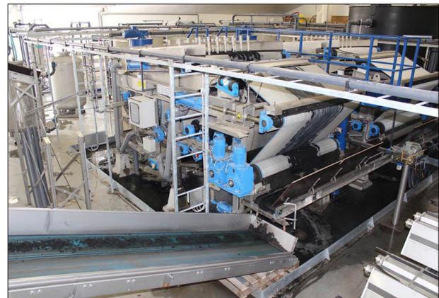
*Slurry and fermentation residues produced in the biogas process can be processed into water, fertiliser concentrate and valuable solids in a four-stage process using the Kumac treatment technology. This process offers a viable, scalable solution, especially in the current situation where high energy costs are leading to sharply rising fertiliser prices and a significant decline in supply.*
