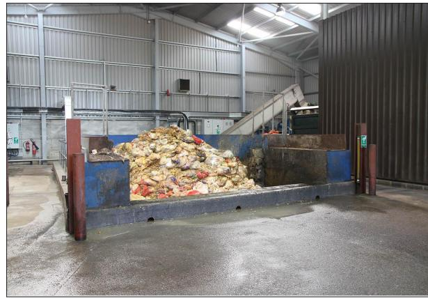
*A WELTEC plant in Piddlehinton, South West England, demonstrates how these goals can be reached with organic waste. Here, a mix of food leftovers, expired food from supermarkets and biowaste is fed into the biogas plant. Apart from the substrate mix, the technical approach, too, is special. Prior to the feed-in and shredding, an unpacking machine separates the food from the packaging.*
