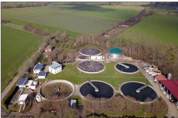
*Until now, the sewage treatment plant with a capacity of 33,000 PE (population equivalents) has applied aerobic wastewater treatment. The conversion to anaerobic sludge stabilisation will put the entire plant on track towards economic and ecological success.*
