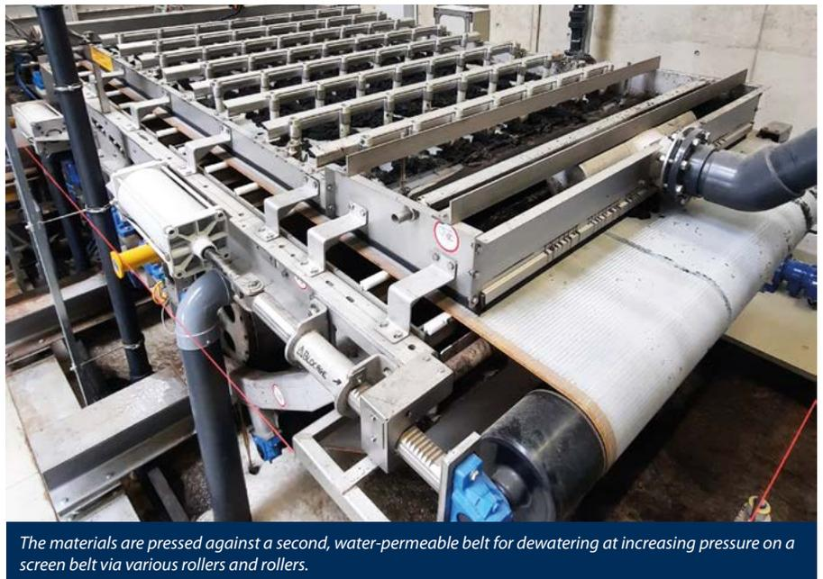
The materials are pressed against a second, water-permeable belt for dewatering at increasing pressure on a screen belt via various rollers and rollers.
